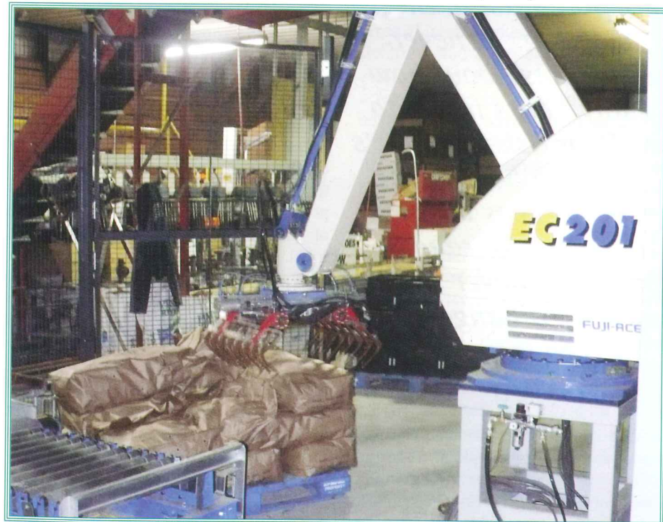
The Fuji-Ace Robotic Palletizer lifts a 50-pound bale of potatoes and stacks it on a pallet at Hamerski Farms, Inc., Plover.
